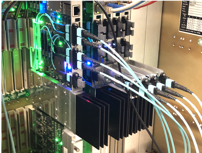
Figure 7.10. The test setup for measuring the optical link quality of the TREX modules. The leftmost module is the transmitter device under-test. It is connected with four fibre ribbons to the four modules on the right, which act as receivers.
