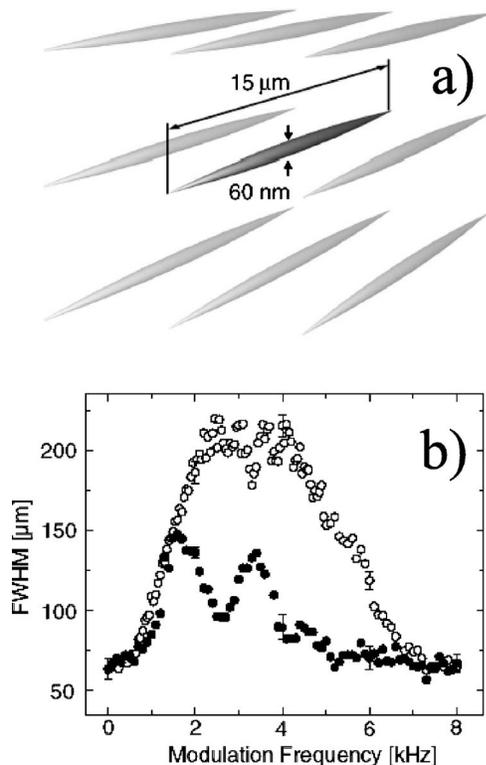
FIG. 27. (a) An array of “tubes” created by a two-dimensional optical lattice, as used in the experiment of Stöferle *et al.* (2004) to realize the Mott-insulator transition in one dimension, and (b) the excitation spectrum of the 1D Mott insulator. The spacing between adjacent tubes in (a) is 413 nm. Taken from Moritz *et al.*, 2003 and Stöferle *et al.*, 2004.
