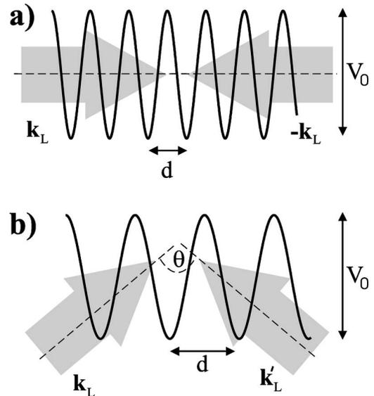
FIG. 1. A one-dimensional optical lattice created from counterpropagating laser beams (a) and with beams enclosing an angle  $\theta$  (b). The parameters  $V_0$  (lattice depth) and  $d$  (lattice spacing) are defined in the text.
